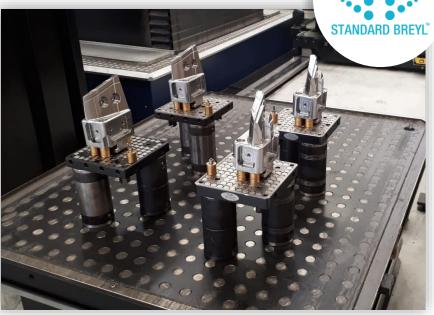
The modularity allows you to create configurations for each machining process giving also the possibility to **recover** the **deformation after heat treatment**
