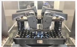
The modularity allows you to create configurations for each machining process giving also the possibility to **recover** the **deformation after** heat treatment
