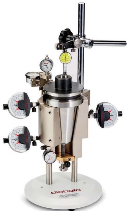
**Taper Gauge for 7/24 Tapers (Steep Taper)**
