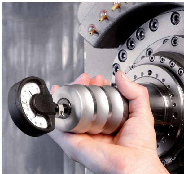
**Mechanical Pull Force Gauges**
