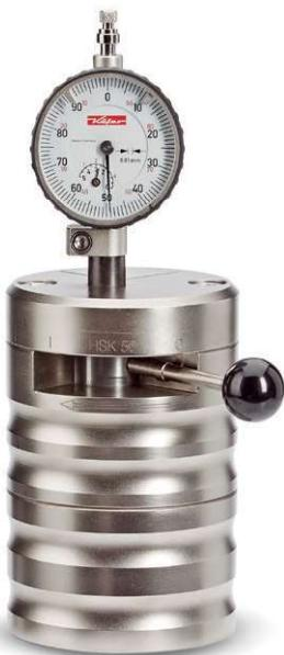
**HSK Tool Holder Cam Angle Gauges
